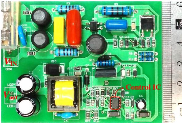
Fig. 14. Prototype of the proposed LED driver.
