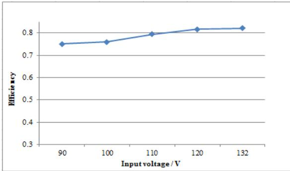
Fig. 17. Measured efficiency versus the ac input voltage.
