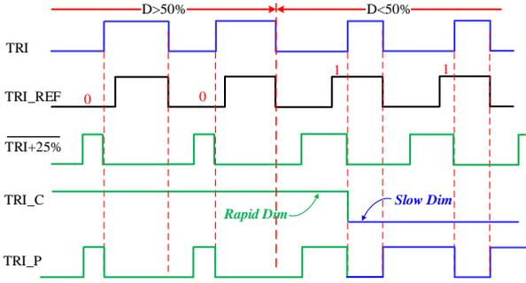
Fig. 11. Key operation waveforms of the switch circuit.
