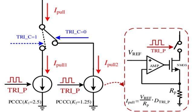
Fig. 12. Design implementation of the pull-down current control circuit.
