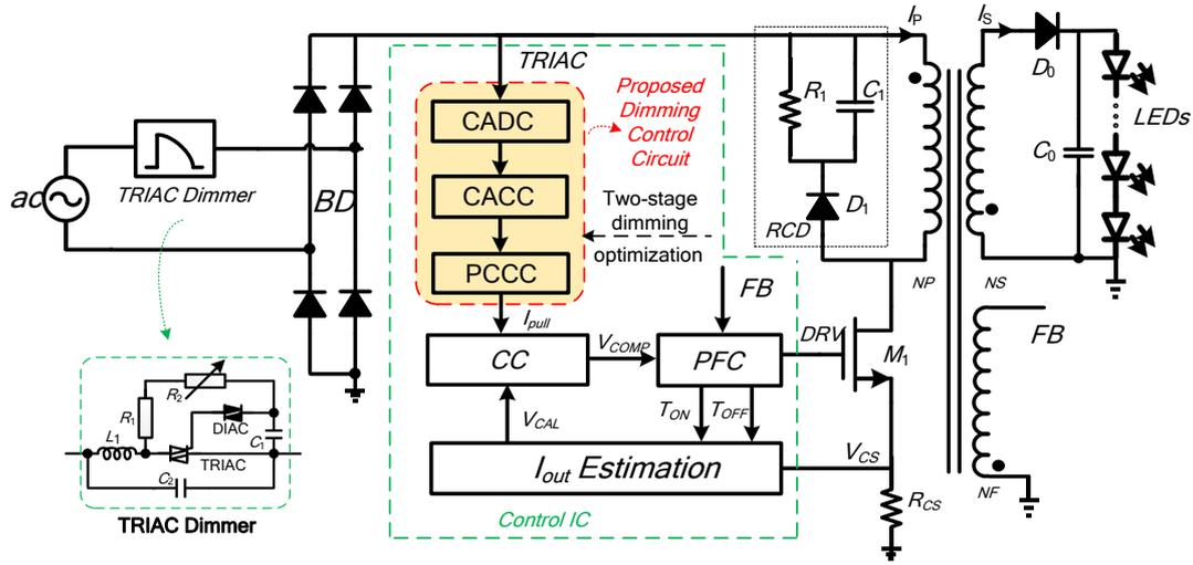
Fig. 1. System diagram of the proposed circuit.
