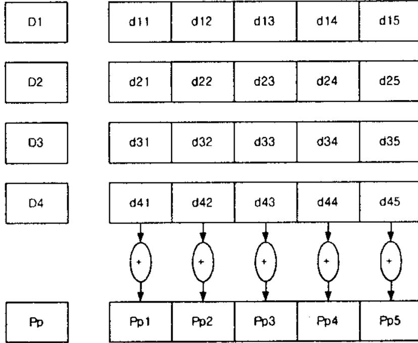
Fig. 3. Vertical Parity Formation Schematic
