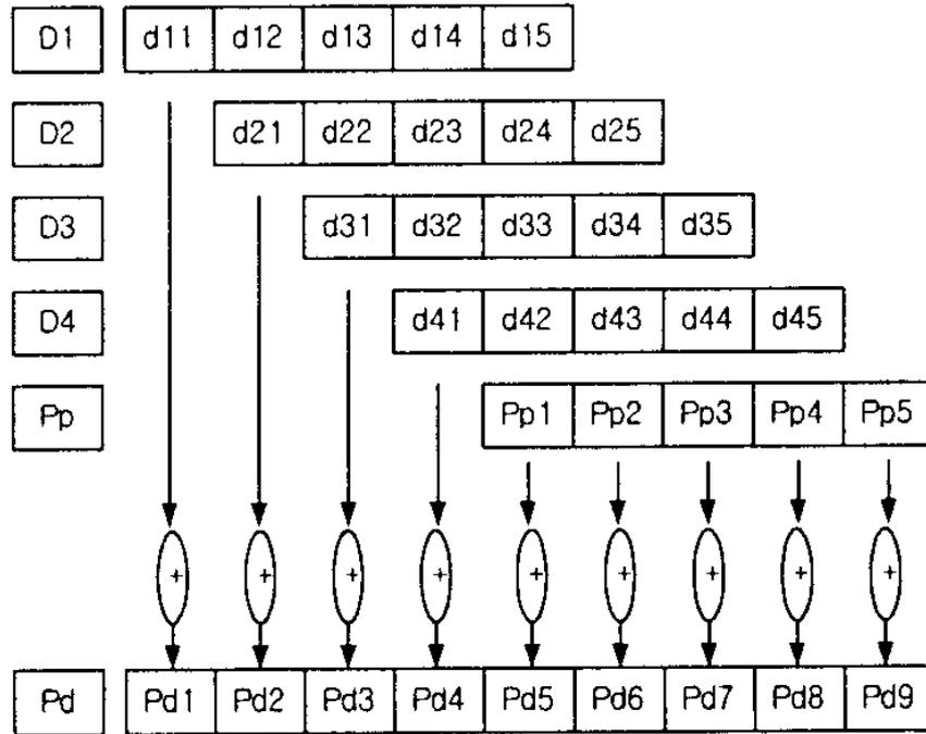
Fig. 4. Diagonal Parity Formation Schematic
